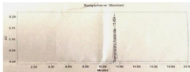
Fig 1: chromatogram of triamcinolone acetonide for trail-1 Trial: 2: Mobile phase :( 70:20:10% Water:Methanol: ACN)
